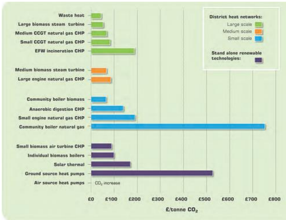
Figure 22: Implied carbon abatement cost (£/tCO 2 for various district and renewable technologies (Source: ZCH, adapted from Pöyry/AECOM & DECC 2009)
